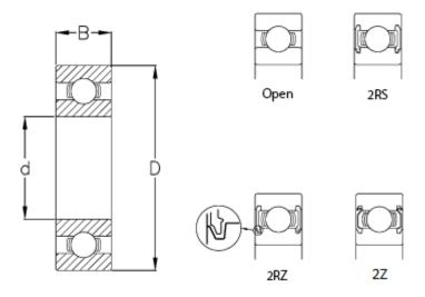
B = 18 Ball grade = 5 C (KN) = 32.5 C0 = 19 d = 40 D = 80 Max rpm. = 14000 Type = 6208
